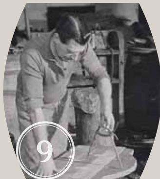
9 Using the 'compass' to measure the heads, which were made from several planks slotted together
