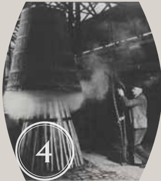
4 Lowering the 'steam bell' over the cask to soften the wood for bending
