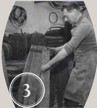
3 'Raising up' the cask by standing the staves upright inside a metal hoop and roughly fixing them together
