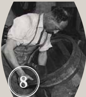
8 Cutting the groove with the 'croze' – ready to fit their two end panels, known as 'heads'
