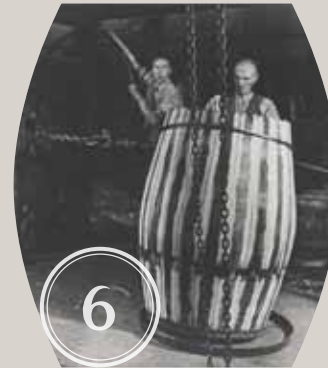
6 Bending the stave ends together and quickly hammering down hoops to create the curved cask shape
