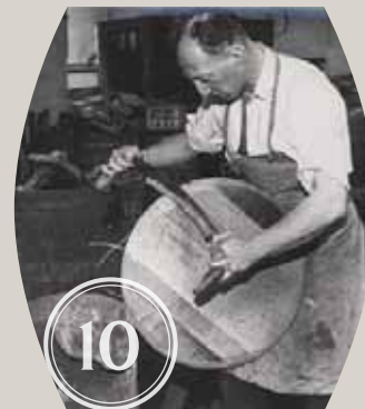
10 Bevelling the edges of the head – a piece of 'flag' (rush) was inserted to help ensure a watertight fit
